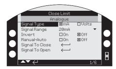
When analogue control is selected independent deadband and hysteresis adjustments are provided in the menu to optimise the control to suit the process conditions. The position against demand profile can also be tailored to suit the specific valve flow characteristics such as linear or equal percentage profile by utilising the Rotork Insight 2 software.
