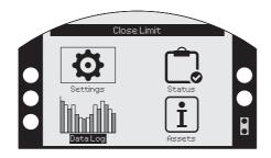
The data can be viewed locally on the dot matrix display and can display graphs of position and pressure through to statistical operational data. All held data is secure and can be downloaded using the Rotork Bluetooth® Setting Tool *Pro* for viewing on a PC with Rotork Insight 2 software.
